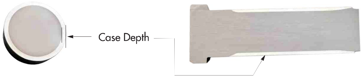
Hardness VS Case Depth Relation - Induction Hardening
