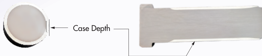
Hardness VS Case Depth Relation Induction Hardening
